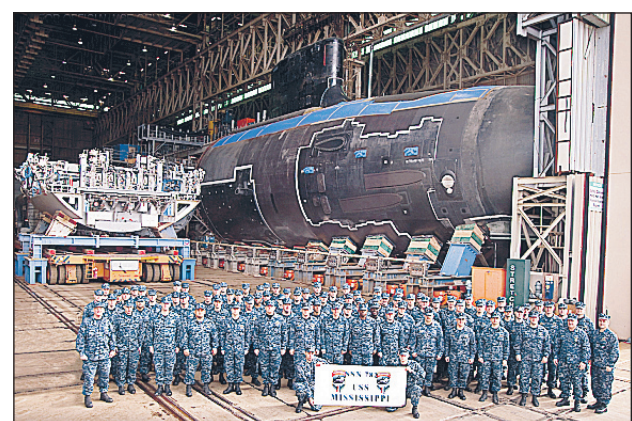
COURTESY GENERAL DYNAMICS ELECTRIC BOAT The sub's crew stand in front of the weapons-handling module, left, before it is inserted into the USS Mississippi, right, at the main assembly building at General Dynamics Electric Boat's shipyard in Groton, Conn.
